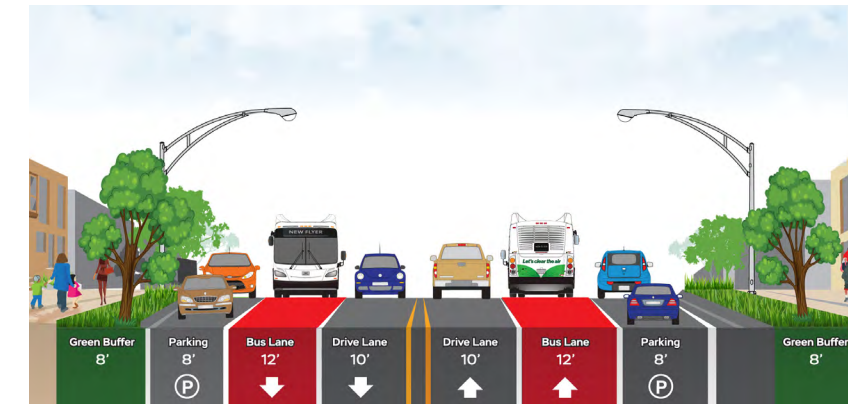
Figure 58 Typical configuration for the middle of the corridor and west of Coppin State University
